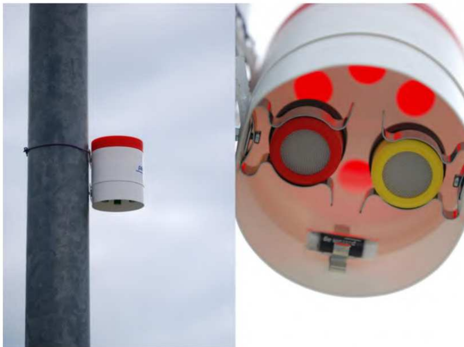
Figure B.5 — Badge-type sampler installed using a protective shelter
